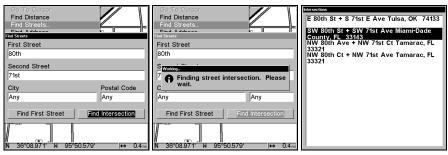
Find Intersection command highlighted, left, and "Working" message, center. At right is the Intersections Found list.
